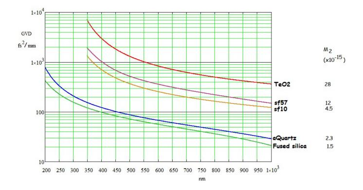
The  $M_2$  figures on right hand vertical axis = the AO figure of Merit at ~1um.
